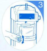
With the switch turned on, receive the shaving with a cup or cone.
